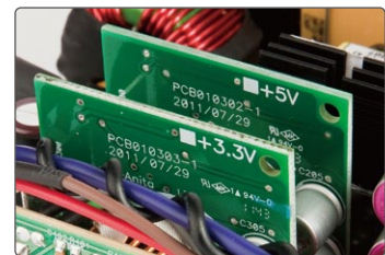
DC-to-DC Converter Design ensures system stability
