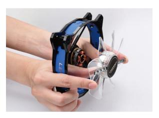
One click to disassemble the fan blades and frame for convenient cleaning.
