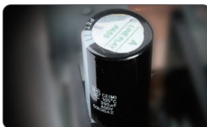
High quality 105°C Japanese-made capacitors
